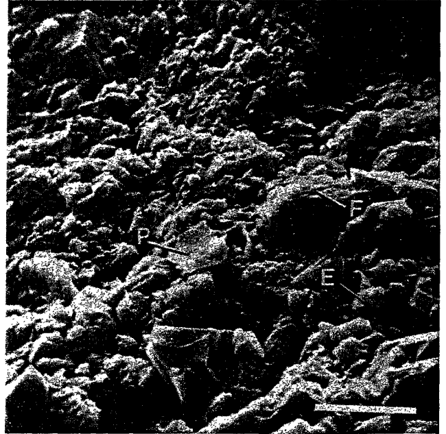
Fig. 14: Fragments of plagioclase (F) in a matrix of equidimensional (E) and platy (P) kaolin particles. Discoloured granite, Hingston Down. Scale bar 10 \mu\text{m} .
