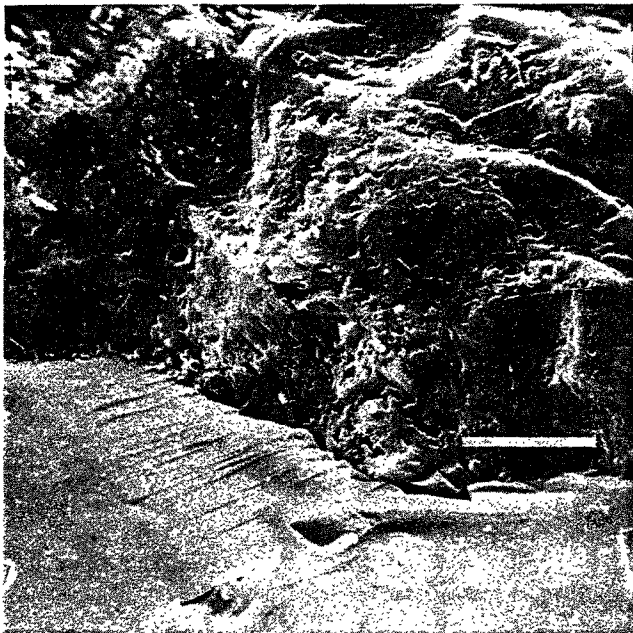
Fig. 5: Prismatic etch pits (PEP's) penetrating potash feldspar. Slightly discoloured granite, Hingston Down. Scale bar 10 \mu\text{m} .
