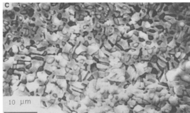
Fig. 8—Morphologies of three Ni-32.5 wt pct Sn eutectic alloy samples with different initial undercoolings. Undercoolings: (a) 31 K, (b) 140 K, and (c) 225 K.
