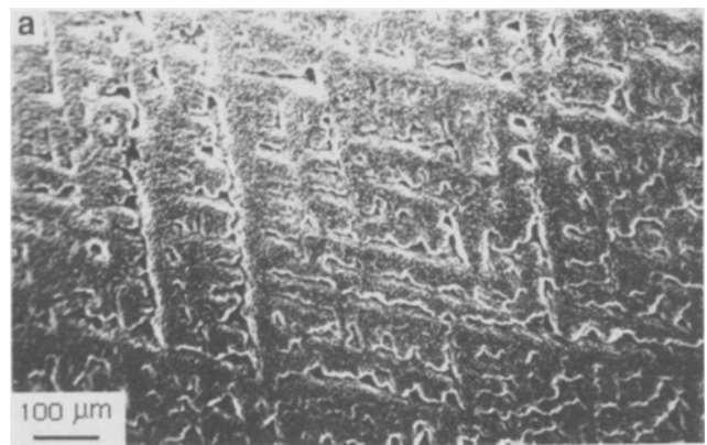
Fig. 9—Well-oriented two-phase dendritic structure observed on the surface of a Ni-32.5 wt pct Sn eutectic alloy sample undercooled 220 K.
