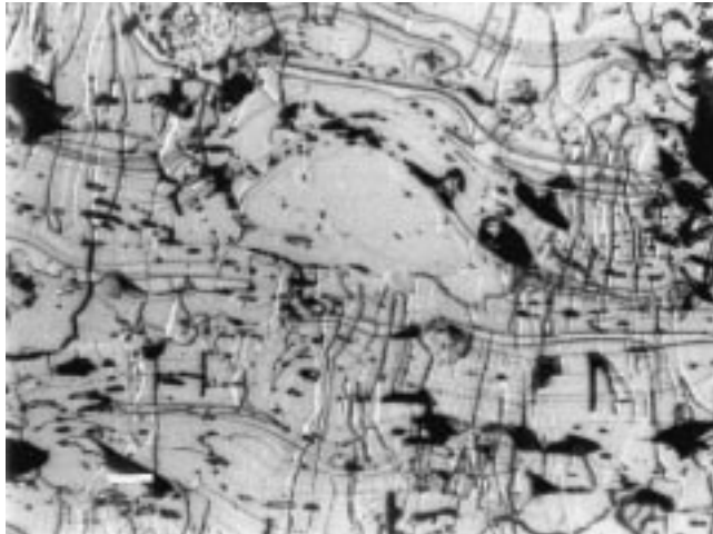
Fig. 22 Microstructure deposited at Ar/H 2 = 120/10 L/min, Z p = 8 cm, Z s = 22 cm, chamber pressure 200 Torr, and particle size -75 μm (deposited partially melted particle on center)
