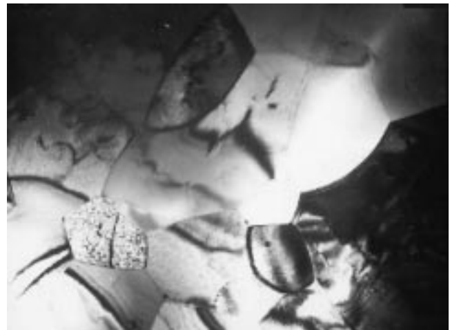
Fig. 17 Microstructure of the initial stage recrystallization (deposition condition: particle size \sim 75 \mu\text{m} , \text{Ar}/\text{H}_2 = 120/20 \text{ L/min} , Z_p = 8 \text{ cm} , Z_s = 30 \text{ cm} , and chamber pressure 200 Torr)
