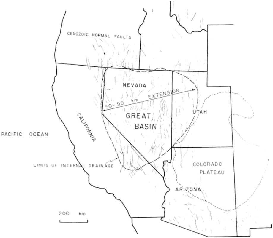
FIG. 1 - Cenozoic normal fault pattern in the western United States. The heavy dashed line delineates the extent of internal drainage that defines the Great Basin. The Colorado Plateau is bordered by the lighter dashed line. Approximately 50 to 90 kilometers of crustal extension is recorded in displacements in surficial Cenozoic normal faults across the Great Basin. Modified after GILLULY (1963).
