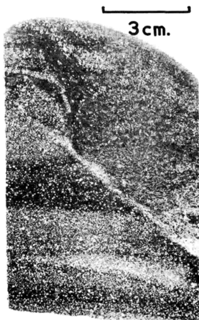
FIG. 11 - Wash-out structure in layered Benfontein kimberlite (specimen S. 14). The layered kimberlite is truncated by structureless calcite-rich kimberlite which contains rafts of the banded kimberlite.
