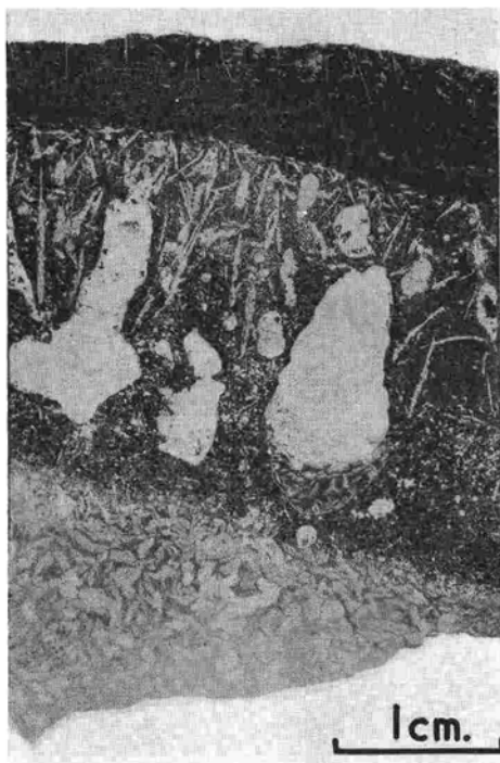
FIG. 8 - Layered Benfontein kimberlite (specimen S. 4b) showing platy calcites (lower layer), calcite-filled migration amygdales, and dendritic calcites.
