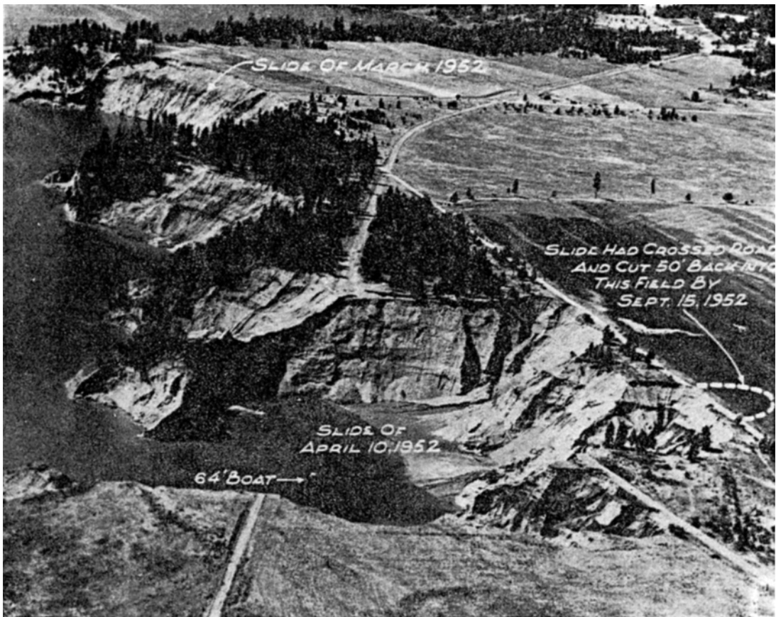
Fig. 13: Shoreline of Figure 12 as it looked on August 1, 1952. The landslide of April 10, 1952, involving about 11 million m^3 , took place by progressive slumping, liquefaction, and flowing of Pleistocene glaciofluvial sediments through a narrow opening (from Jones et al. 1961; Varnes 1978). (Photograph by F. O. Jones, U. S. Geological Survey.)
