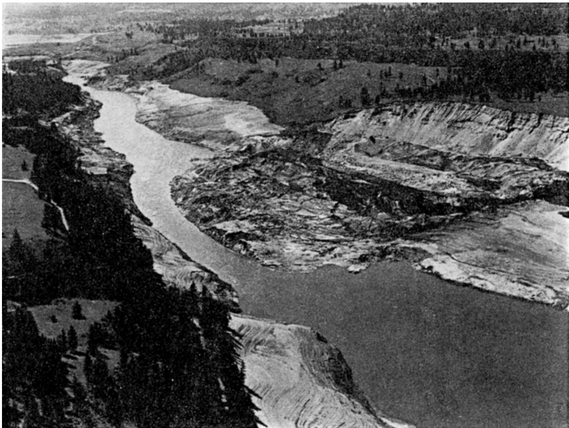
Fig. 14: Jackson Springs slide on the Spokane arm of Roosevelt Lake. This earth slump, which had a volume estimated at over 11 million m^3 , occurred on March 26, 1969, on a terrace consisting of alternating beds of lacustrine clay, silt, and sand. The slump occurred during a period of extreme drawdown necessitated by excavation for a forebay dam preliminary to construction of the Third Powerplant at Grand Coulee Dam (U. S. Bureau of Reclamation 1969). (Photograph courtesy of U. S. Bureau of Reclamation.)
