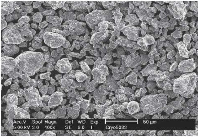
Fig. 2—Secondary electron SEM image showing the morphology and size of the cryomilled 5083 Al powder.
