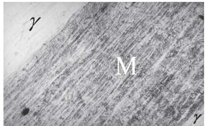
Fig. 7—Martensitic layer surrounded by austenite phase.
