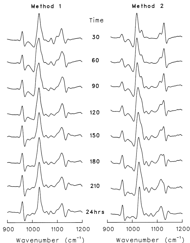
Fig. 2. Second-derivative spectra of the \nu_1 , \nu_3 phosphate region of the HA synthesized by method one and method two as shown in Figure 1. In method one, the pH was fixed at 7.4. In method two, the pH was allowed to vary throughout the reaction. Times (minutes) shown are the times when the aliquots were withdrawn.
