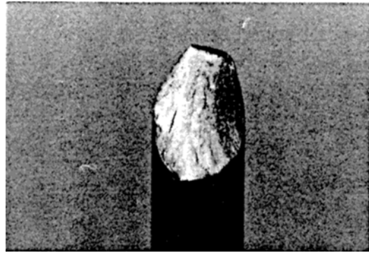
Fig. 4 Tests at \dot{\epsilon} = 10^{-5} \text{ s}^{-1} . (System 1) Fracture initiated at an indentation produced by the wedge. Shear fracture.
