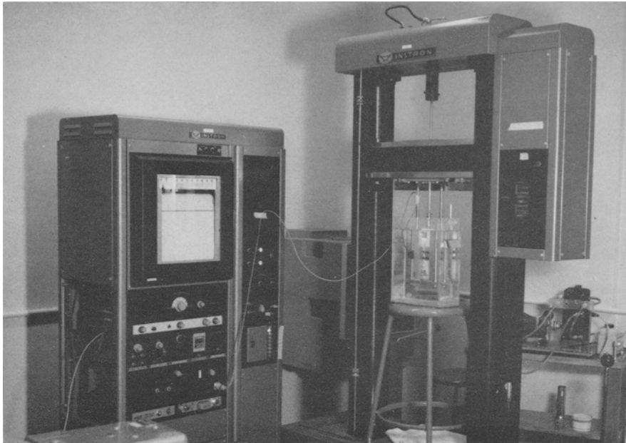
FIG. 1. Instron Tester. Control console is on the left and crosshead assembly is on the right. The clear plastic tank is placed below the crosshead so that the tendon specimen can be immersed in Ringer's solution.
