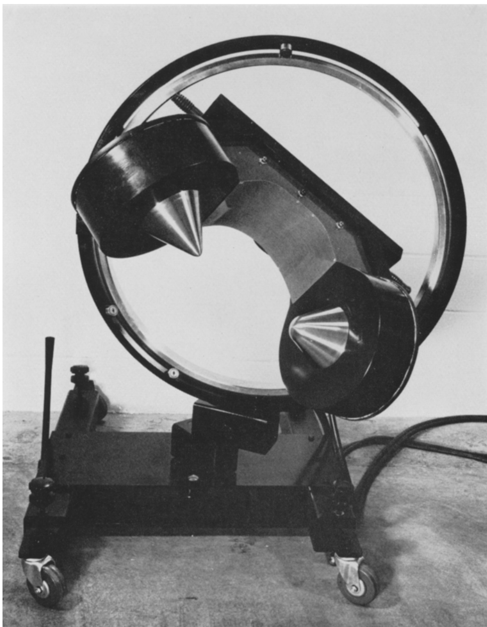
FIG. 1. Five kW electromagnet and mounting which permits horizontal translation and rotation about three axes.
