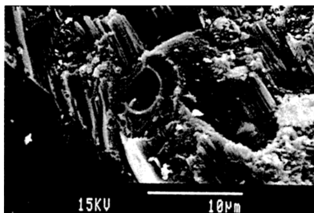
Fig. 13 The interfacial zone in cement-30% fly ash-gypsum mortar.
