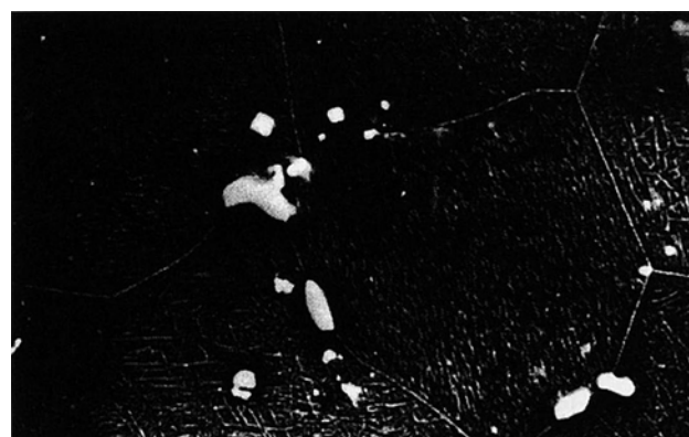
Fig. 4. Microstructure of alloy WE43 in heat-treated state, \times 1500 .
