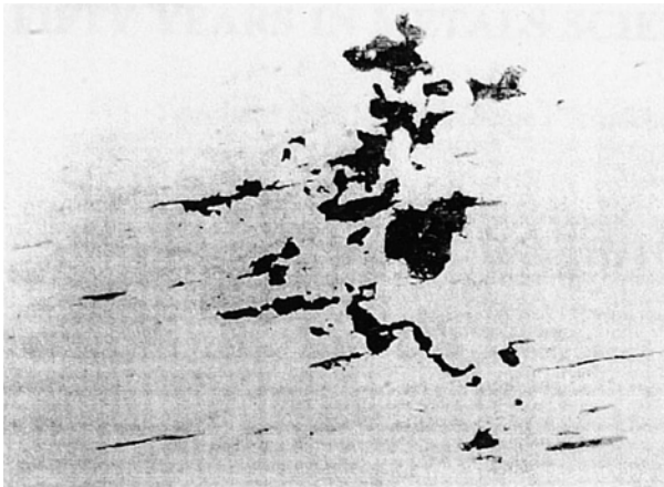
Fig. 2. Nonmetallic inclusions (sulfides) in imported steel AS45G2 ( \times 400 ).
