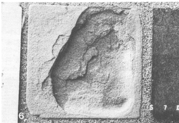
Figure 6. Weathering of sandstone by scaling. Migration of grain cement from inside to the surface, migration also from mortar joint. Specimen is 10 cm long. National Bureau of Standards Stone Test Wall.
