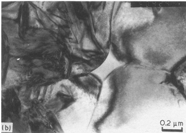
Figure 4 Two transmission electron micrographs showing the occurrence of a glassy phase at grain boundaries and junctions in the sintered material (8 h). The glassy phases are due to the high silica impurity in the electrorefined ZrO_2 powder. It is believed that the occurrence of such a liquid phase at sintering temperature assists the densification of zirconia ceramics. However, the resultant glassy phase at grain boundaries and junctions will suppress the autocatalytic nature of the transformation.
