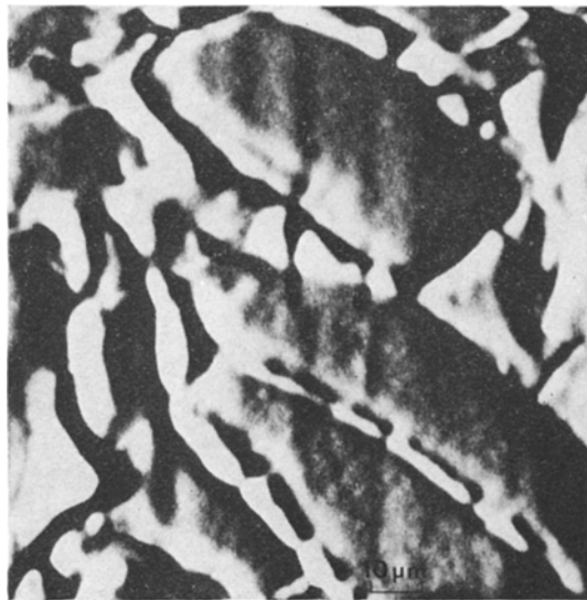
Figure 8 Electron back-scatter image photograph of cement C-2 prepared for EPMA study.
