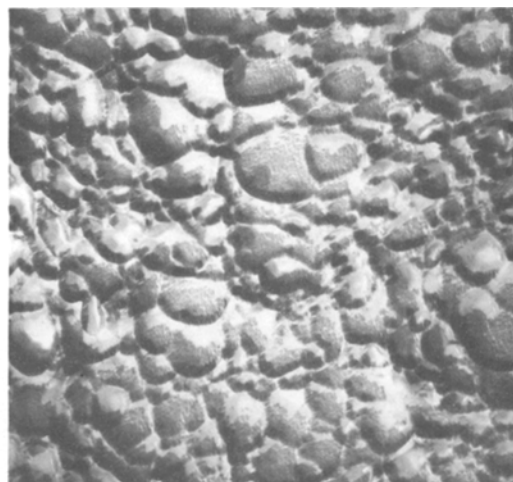
Figure 4 Electron micrograph from two-stage replica of hydroxylapatite fired 1 h at 1000^\circ\text{C} (C-2), \times 33\,000 .
