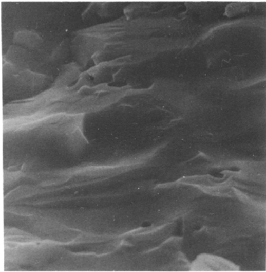
Figure 3 Scanning electron micrograph of static torsion fracture surface of hydroxyapatite sintered at 1300°C for 3 h showing transgranular fracture ( \times 3000 ).
