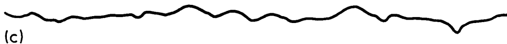
Figure 8 The surface structure of the bottom of a solidified tin drop that had been in contact, at 500^\circ\text{C} , with the silica surface illustrated in Fig. 7, as revealed by (a) and (b) scanning electron microscopy ( \times 36 ) and ( \times 145 ) and (c) surface profilometry ( \times 2500 vertical) and ( \times 100 horizontal).
