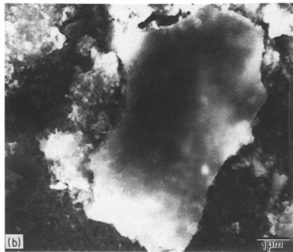
Figure 5 Representative SEM micrograph showing: (a) the fractured surface of the as-deposited Al-Li-SiC p , and (b) the presence of reaction products in the remelted Al-Li-SiC p material (Ht3 condition).
