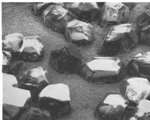
Figure 7 Scanning electron micrograph of the surface of a diamond grit copper-0.73% titanium alloy compact, produced by hot-pressing for 5.0h at 700°C, used to abrade steel sheet for 0.5h, 60°C, \times 120 .
