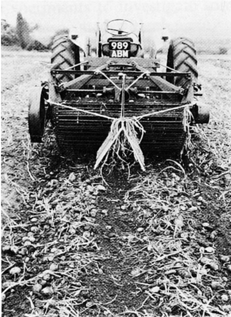
Fig. 2. Fixed share two row digger with divider.
