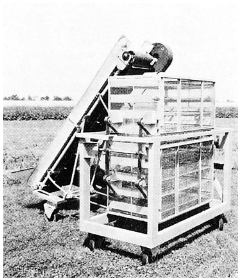
Fig. 6. N.I.A.E. Multi-grade potato riddle.
