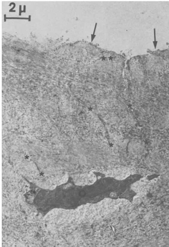
FIGURE 9. Decalcified bone tissue from the interface (arrows) zone of a titanium implant after 5 years of clinical function. An osteocyte (O) with processes (*) penetrating in the direction of the interface. The collagen in a two micron wide zone (***) close to the implant is less regularly organized in comparison to the deeper parts of the tissue.
