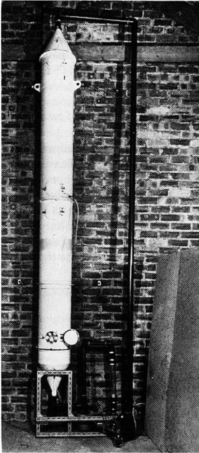
Fig. 2. Cylindrical fumigation chamber. Bottom port is open.
