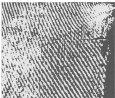
Fig. 7(b)—Binarization of fringes in Fig. 4
