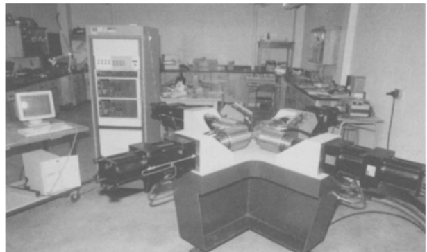
Fig. 3—Photograph of the biaxial testing apparatus
