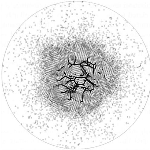
Fig. 2. A snapshot from an event-driven molecular dynamics simulation of 5000 hard spheres. The wall is kept at a fixed temperature. The gray scale codes the relative number of collisions experienced by particles during the previous  $10^5$  time steps. One distinguishes three regions: a gaslike state with low density, and two high-density regions, with and without collision chains (cf. Fig. 1).
