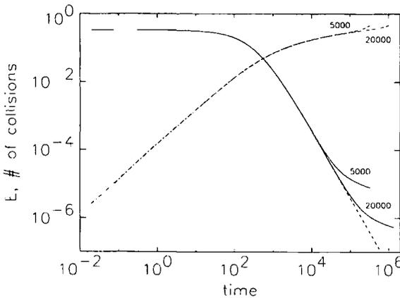
Fig. 3. The kinetic energy  $E$  per particle over time  $t$  from MD simulations. Energy decay curves for systems with 5000 and 20,000 particles are identical for a very long time (solid lines). The dashed line shows the prediction of Eq. (8) with  $T_0 = 0.333$  and  $A = 0.01$ . The dash-dotted lines display the cumulative number of collisions per particle scaled by factors  $10^{-8}$  (5000) and  $4 \times 10^{-8}$  (20,000).
