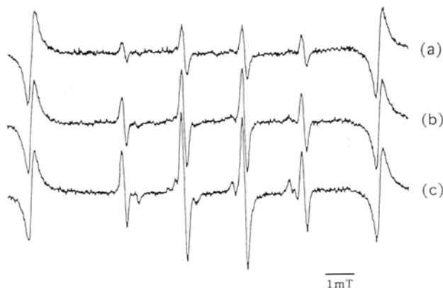
Fig 3. Electron paramagnetic resonance (EPR) signals of the DMPO-OH spin adduct obtained from neutrophils stimulated by H. pylori extract. Tracing a: 1 min after the addition of H. pylori extract; tracing b, 6 min after the addition of H. pylori extract; and tracing c, 11 min after the addition of H. pylori extract. These EPR tracings show one of the three experiments.
