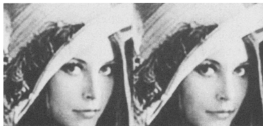
Figure 9. Comparison of the reconstructions obtained with the Cortex Transform, CT (a), and the Gaussian Wavelets Transform GWT (b). In both cases, the peak frequencies and orientations are the same, and the high frequency residual has been neglected.
