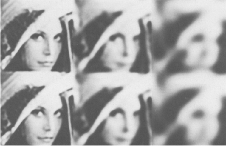
Figure 10. Image reconstructions with partial losses of frequency channels. The first row (up) corresponds to the CT and the second (down) to the GWT. The first column (left) shows the reconstruction from only three frequency channels (missing the high frequency channel), and the second and third columns to reconstructions from two and only one channels, respectively.
