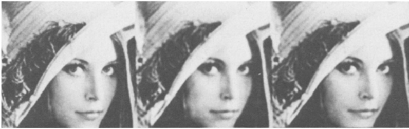
Figure 8. Original image (a) and reconstructions from Fourier domain (b), and spatial domain (c) implementations of the GWT.
