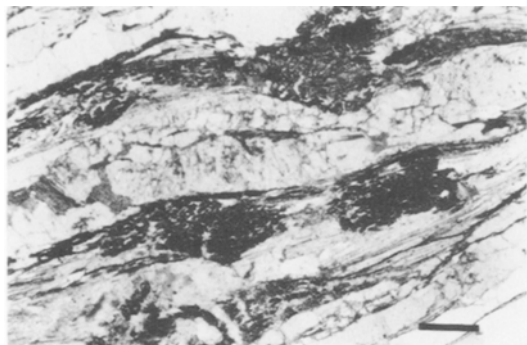
Fig. 2. Relic kyanite in the S2 foliation. Kyanite is boudinaged in the S2 foliation, shows undulose extinctions and is retrogressed into muscovite (scale bar = 0.5mm).
