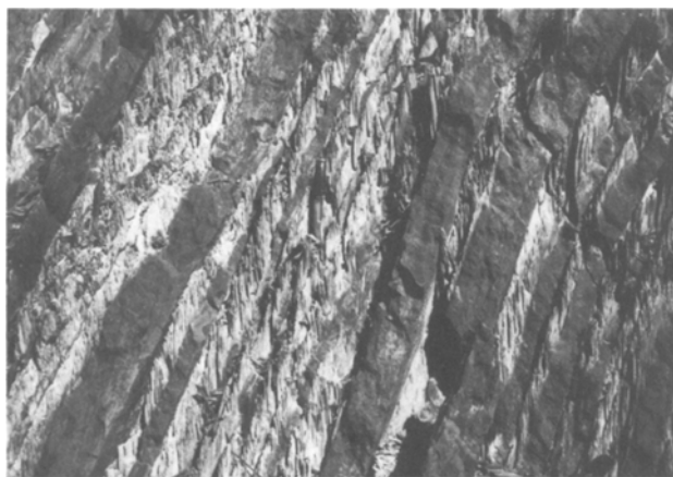
Fig. 2. Bedrock consisting of flysch in Makran. Even in imperious rocks, the hydraulic permeability is much higher when they are tectonized. The figure clearly shows fracture cleavage in vertical direction suggesting strong lateral pressure. Although the cleavage does not pervade the sandstone interbeddings, combined with a fault, the permeability of the whole rock increases considerably.
