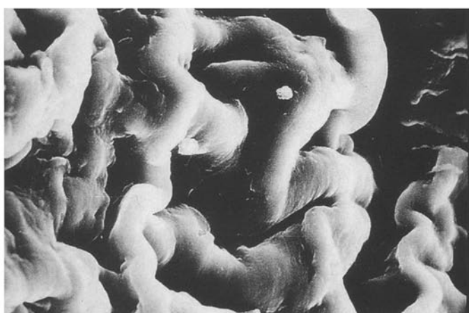
Fig. 13. Scanning electron microscopic view of (superficial) femoral a. (x1000). Note that the vascular endothelium was not damaged by testing in our mock circulation loop
