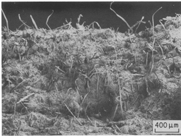
Figure 3 Uneven fracture surface of WFRP (4% fibre by mass), suggesting considerable increase in fracture energy.
