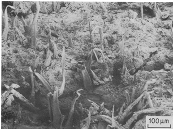
Figure 4 High magnification of WFRP fracture surface, showing fibres both fractured and pulled-out from the matrix.
