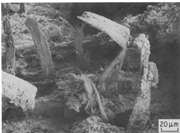
Figure 5 Fibres failed in tension with some showing “buckling”.
