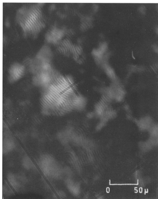
Fig. 2. Polarized light optical photomicrograph of HPC in acetic acid at 0.325 gm/ml
