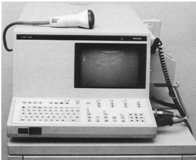
Fig. 1. The Philips SDR-1500 mobile, real-time, B-mode ultrasound scanner and the small parts 7.5-MHz transducer.
