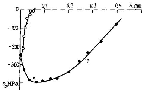
Fig. 1. Curves for axial residual macrostresses in cylindrical specimens of steel 20 after mechanical polishing (1) and SPD (2).
