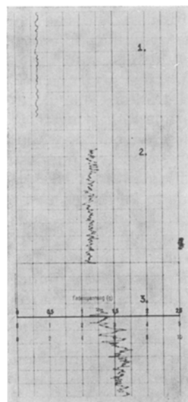
Fig. 16. Tensiometric curves for various systems of fibre leading. 1. - freely running fibre; 2. - fibre tangentially wetted; 3. - fibre led through the leading roll and the wetting disc. (cf. table 2, yarn B)
