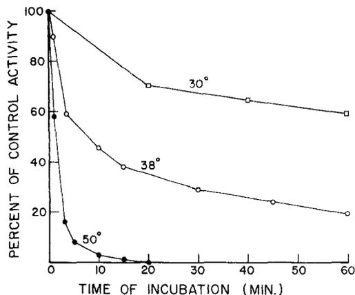
Figure 9. Heat stability of Emasol-treated lipid-depleted cytochrome oxidase. 30 mg Emasol-1130/mg enzyme protein was added before incubation. Control activity as 100% was  $43.2 \mu\text{moles O}_2/\text{min}/\text{mg}$  protein.
