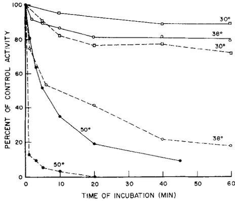
Figure 7. Heat stability of lipid-containing and lipid-depleted cytochrome oxidase. Enzyme was incubated at temperature indicated at protein concentration of 1 mg/ml. 50  $\mu$ g phospholipid phosphorus/mg enzyme protein was added before or after incubation. Solid lines are the lipid-containing cytochrome oxidase; dotted lines, lipid-depleted enzyme with phospholipids added after incubation. Control activity as 100% was 41.2  $\mu$ moles O<sub>2</sub>/min/mg protein.
