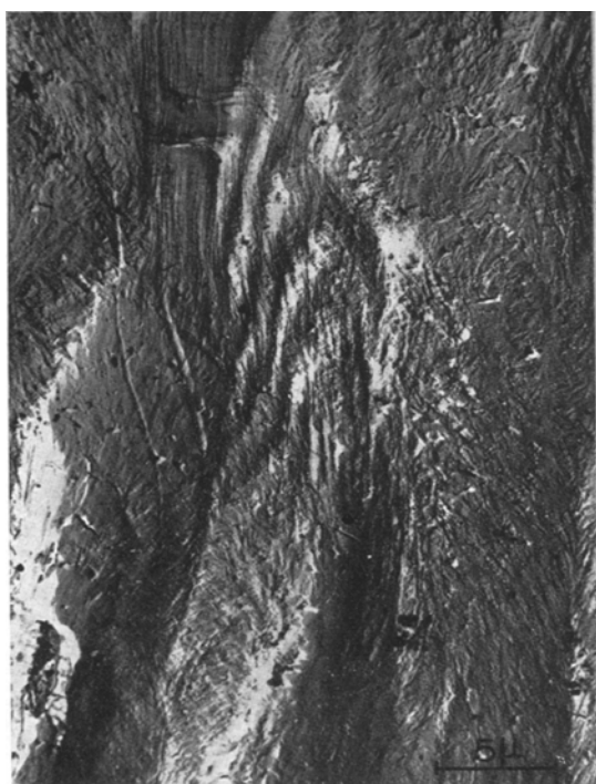
Fig. 32. Highly drawn O.C.P. film. Electron micrograph of two stage replica. (Draw direction vertical)
