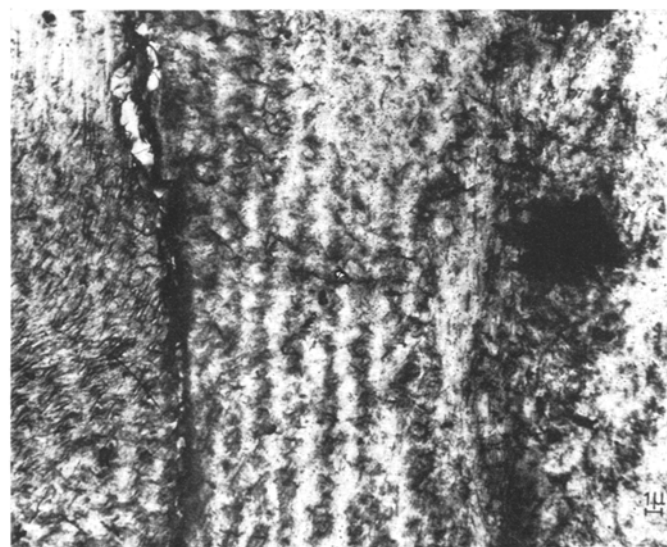
Fig. 35. Enlarged detail of spherulite in fig. 33 showing radii perpendicular to draw direction. (Vertical)
