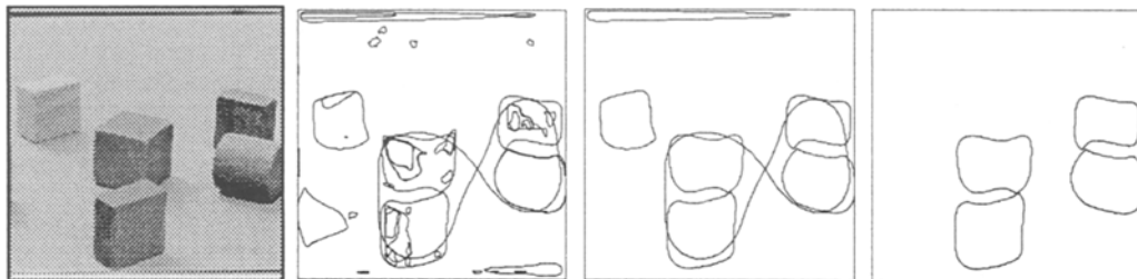
Fig. 14. Boundaries of the dark scale-space blobs extracted from the toy block image. (Left) Original image. (Middle left) The 50 most significant dark blobs. (Middle right) Low threshold on the significance measure set in one of the “gaps” in the sequence of significance values (between 74 and 131). (Right) High threshold on the significance measure set in another “gap” (between 298 and 591). (The significance values are shown in table 1.)
