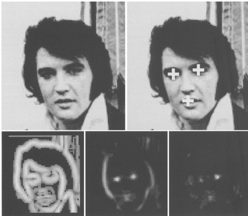
Fig. 5. Further processing the previous figure. Top: Area around the highest radial-symmetry peak in finer resolution and the peaks of the radial symmetry. Bottom: Edge detection (left), isotropic symmetry (middle), and radial symmetry (right).
