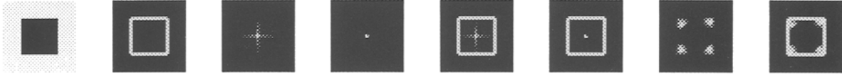
Fig. 11. Applying the symmetry transform on a simple figure. Left to right Original image; its edges; isotropic symmetry with a large \sigma ; radial symmetry with the same \sigma ; superposition of the isotropic symmetry with the edges—the skeleton detected; superposition of the radial symmetry with the edges (compare to previous figure); isotropic symmetry with a small \sigma —the corners detected; superposition of the fine symmetry with the edges.
