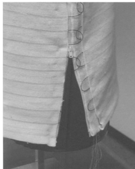
Fig. 9. Zipper attachment on knitted Wearable Motherboard™.
