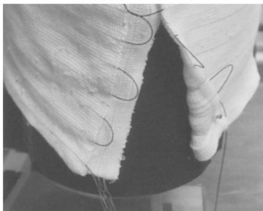
Fig. 8. Velcro attachment on knitted Wearable Motherboard™.
