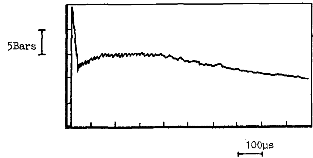
Fig. 14. Example of experimental pressure profile of SFD recorded in an ethylene/air mixture ( r = 1.15 ) with 13 \mu\text{m} aluminum particles ( \sigma = 60 \text{ g/m}^3 )
