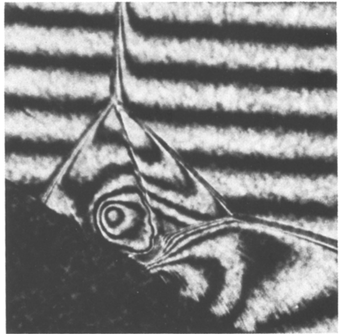
Fig. 7. An enlarged photograph of a DMR illustrating the interaction of the second Mach stem with the first contact discontinuity (courtesy of Prof. I. I. Glass)
