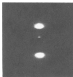
Fig. 3. Small-angle X-ray scattering pattern for oriented nylon-12 (corresponding to TEM image of fig. 1)
