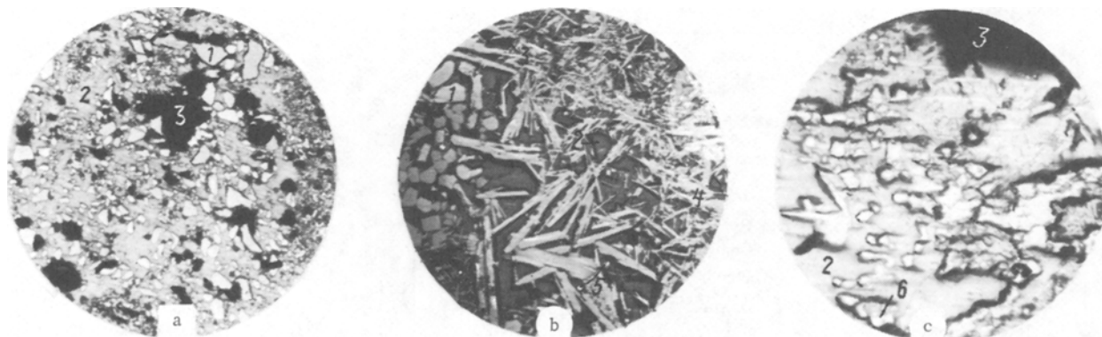
Fig. 3. Microstructure of MKT after service: a) transition zone, b) reaction zone, c) slag skin; 1) corundum, 2) glassy-mullite phase, 3) pores, 4) \beta -alumina, 5) metal, 6) spinel, a, b) \times 100 , c) \times 200 . Reflected light.
