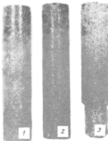
Fig. 4. Specimens after slag testing by rotating in slag: 1) silicon carbide refractory bonded with silicon oxynitride; 2) SiC refractory with a silicon nitride bond; 3) chamotte grade ShPD-41.
