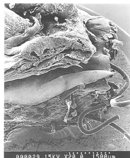
Fig. 4 SEM aspect of the polypropylene – PTFE mesh after three weeks (magnification x 20)
